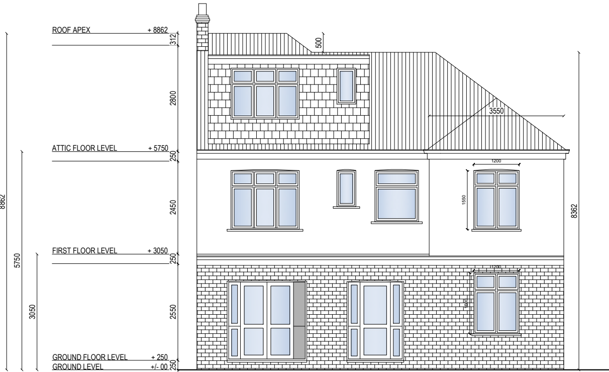
PROPOSED RIGHT-SIDE ELEVATION 1: 100 @A3
